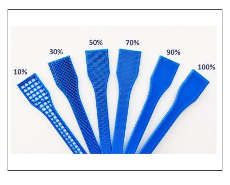
• Infill percent determines what percent of the internal structure needs to be filled directly. The higher the infill, the stronger the print will be, but the longer it will take to print. An average print really doesn't need higher than 15% infill, although certain prints may require more based on what they will be used for.
